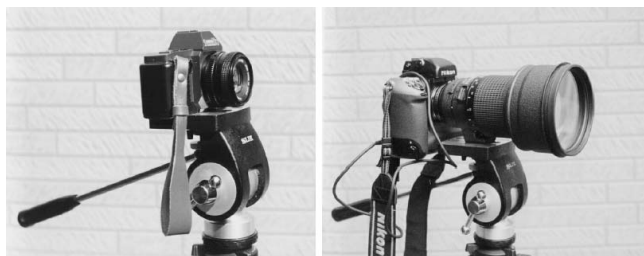
Fig. 3. Typical 35 mm size photographic cameras used for persistent train imaging. Wide aperture lenses were selected for detecting faint luminescence. Equipped lenses are a 50 mm lens of F=1.4 (left) and a 200 mm telephoto lens of F=2.0 (right), respectively. The camera with telephoto lens should be loaded with another sub-camera with a 50 mm lens because wide field of view is effective for determining the direction of field as well as for fail-safe operation. In addition, a steady single-grip and well-balanced camera platform is necessary for quick aiming. A photographic camera with autowinder and data backup system has great advantage for accurate persistent train imaging.
