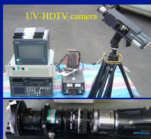
UV-HDTV camera (UV sensitive I.I.-HDTV camera, above) and I.I.-HDTV camera with grism (Direct vision grating, below).
